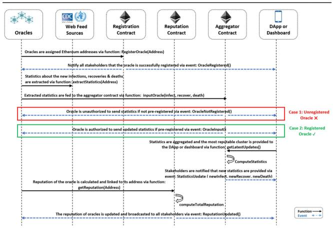
Fig. 4 Sequence diagram showing the function calls and events in a blockchain-based COVID-19 tracking system
